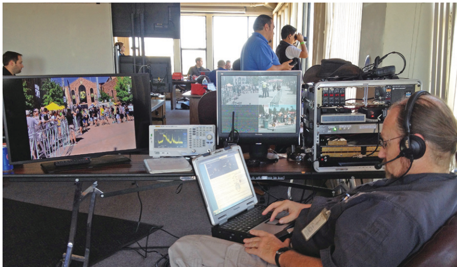
Figure 4 — Inside the Colorado University police command post. Mark Huff, KB0LRS, at the BCARES TV net control position, monitors live (left) digital DVB-T and (right) analog images.
