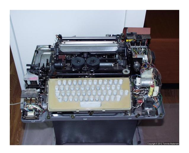
Used a synchronous motor rotating disk and brushes to generate and receive the data
